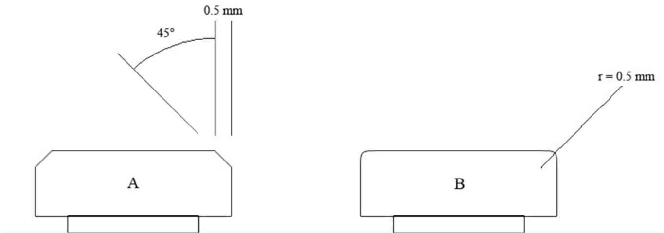
Figure 11. Épée details of tip and point
