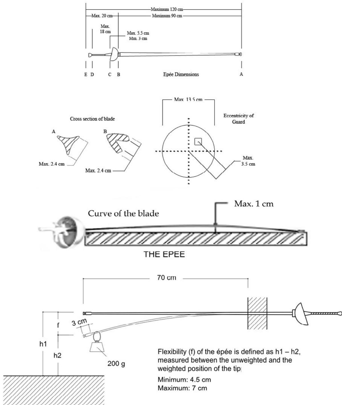
Figure 9. Epée dimensions and flexibility
